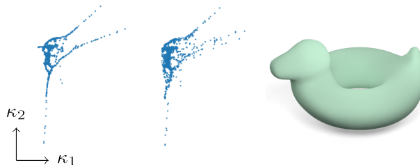
Figure 13: Limitation of shape deformation. Here we show the intermediate output from the last iteration of optimizing an organic shape. From left to right : Principal curvature diagram from curvature diagram transformation, resultant curvature diagram after shape deformation, output mesh.
