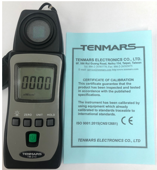
Fig. 1. We show the TENMARS TM-213 UV-AB Light Meter and its CERTIFICATE OF CALIBRATION , respectively.
