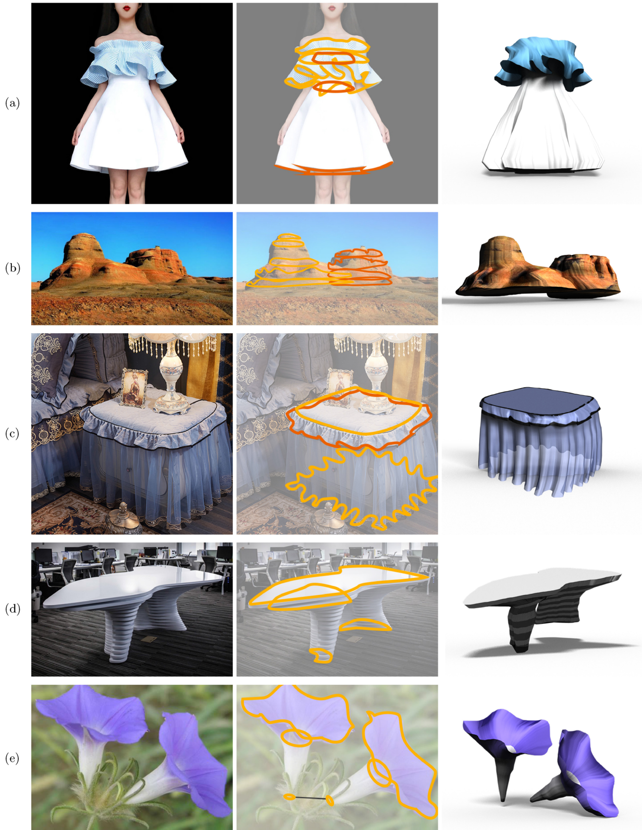
Fig. 8 Modeling lofted shapes with multiple parts. Left: input images. Middle: input curves representing the outlines of cross sections. Right: reconstructed 3D models.
